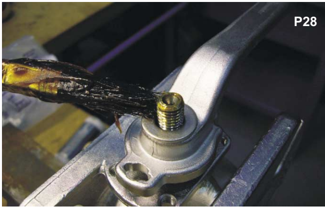
Apply rocol to the spindle thread.
