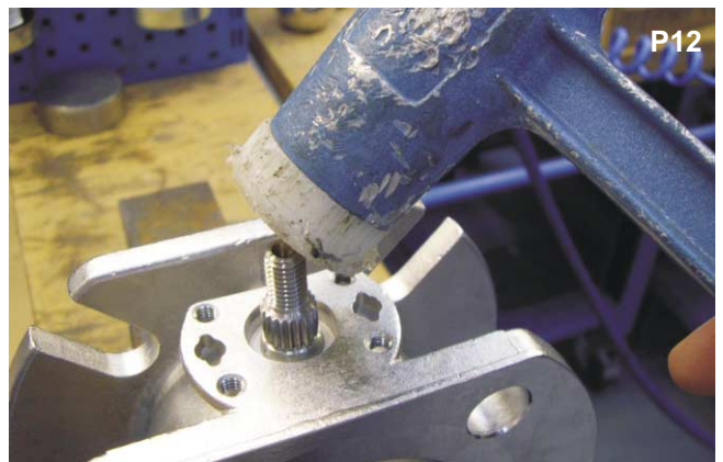
If needed carefully tap the spindle to free from bore.
