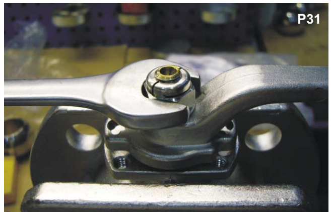
Using a 17mm A/F wrench tighten the lock nut.
