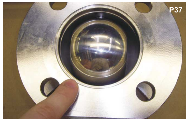
Ensure that the front seal groove is clean and free from any dirt.
